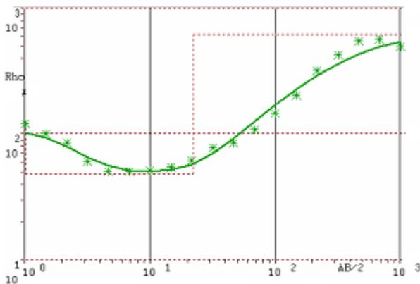
**Figure 4:** Observed and computed VES 1 sounding curve at 500 m point of profile 1.
