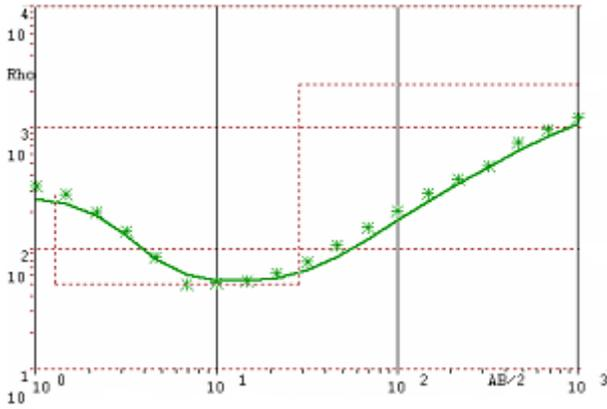
**Figure 5:** Observed and computed VES 7 curve at 640m point of profile 1.
