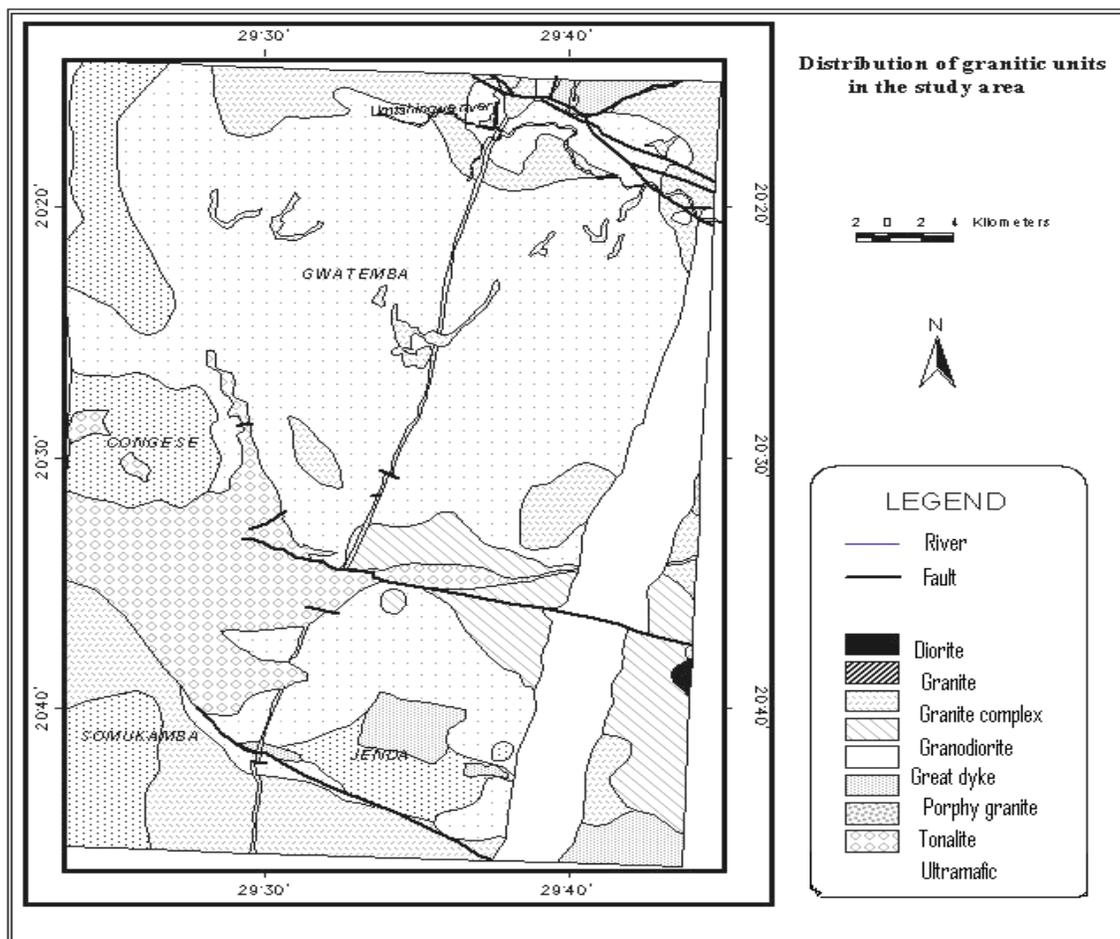
**Figure 2:** Distribution of granitic units in the Gwatemba area (adopted from ‘The geology of the Filabusi greenstone and the surrounding granitic terrain by N. Baglow’).
