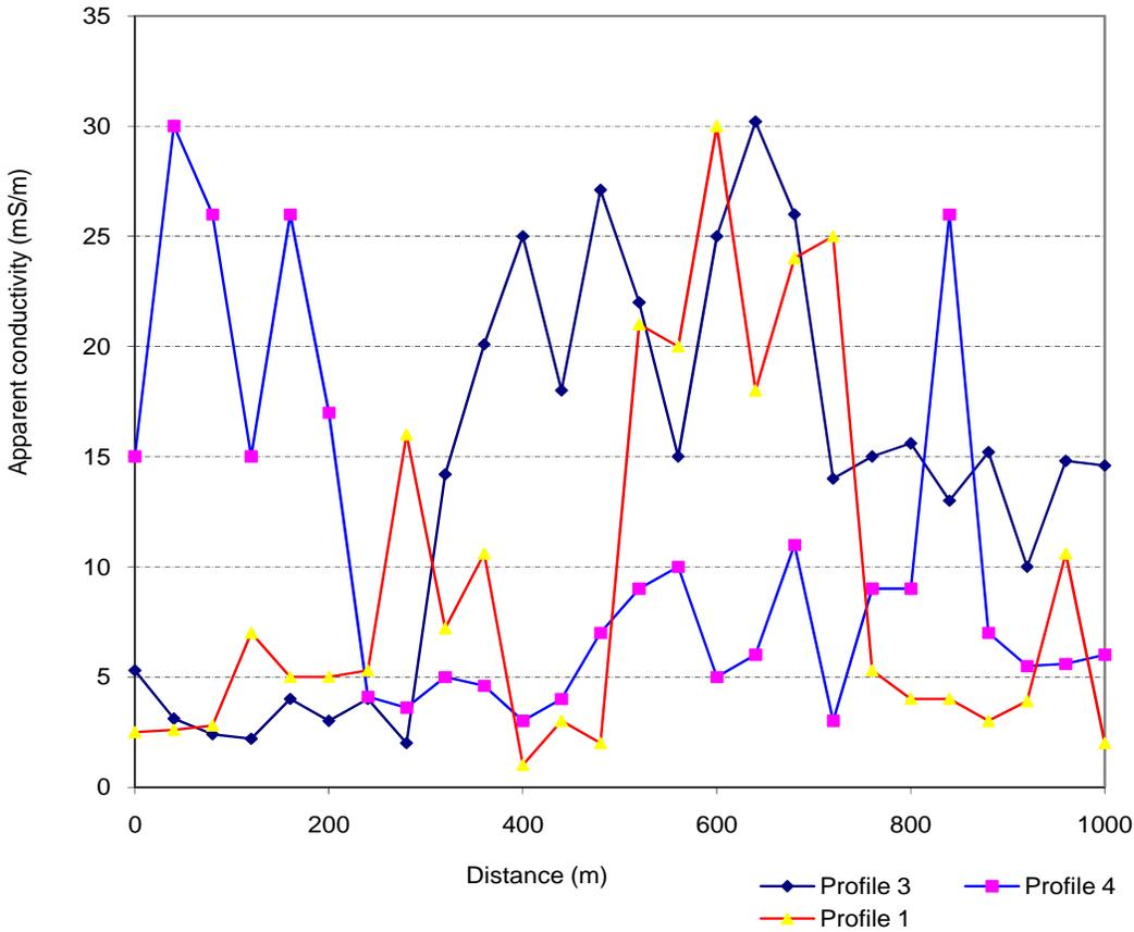
**Figure 3:** Plot of Apparent conductivity data against length of profile line 1, 3 and 4
