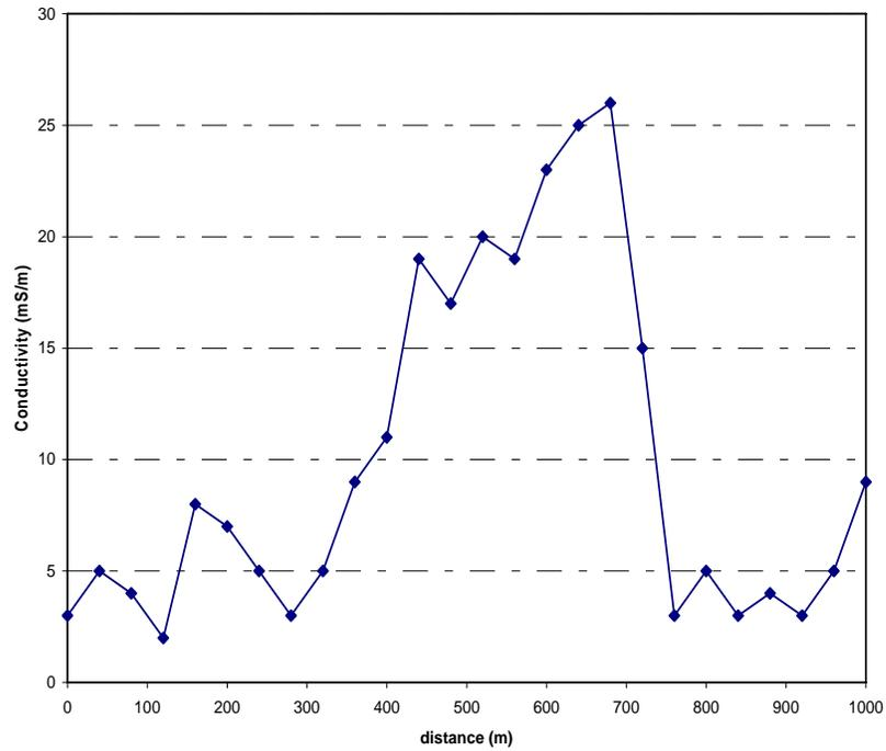
**Figure 2:** Plot of EM34-3 data from profile line 02 in the study area.
